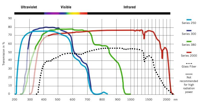
Measured with 2 $\alpha$ =50° (Series 250 2 $\alpha$ =34°), length 2000mm, active core Ø5mm
