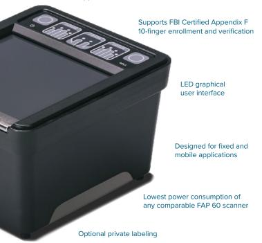
Kojak ends the myth that 4-4-2 FAP 60 fingerprint scanners must be big, heavy, and power hungry. This compact, lightweight unit delivers fast FBI Certified Appendix F performance for 10-print enrollment and verification in a compact form factor that uses less power than any other FAP 60 scanner currently available.
