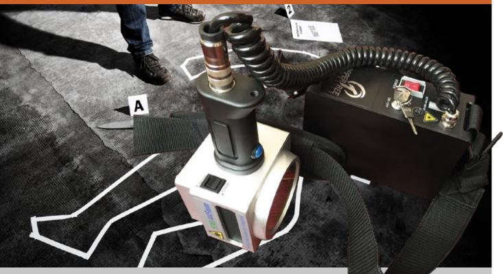
The Disaster Victim Identification - LED (DVI-LED) is a safe and powerful LED light source, for any crime scene, Lab, Fire or disaster location.
