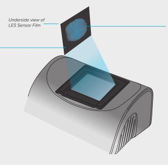
A CMOS camera captures the glow from the phosphor particles, producing a high-resolution fingerprint image
